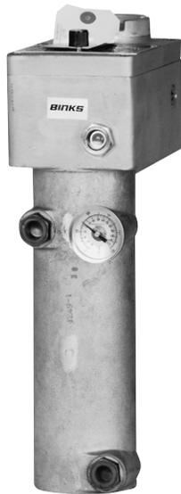
High pressure, lightweight (28 lbs), compact construction. Working capacity to 5000 psi and with adjustable thermostatic control from 60° to 250°F. The typical temperature rise with a flow of 32 fl. oz./min. while maintaining a temperature of 100% above ambient is 100°F. 1/2" npt(f) inlet and outlet ports. (CSA listed, CE approved)
